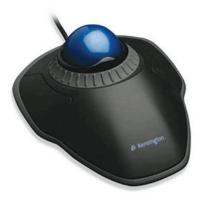
It is a stationary input device that has ball mechanism to move the pointer or cursor on the screen. The ball is half inserted in the device and can be easily rolled with finger, thumb or the palm to move the pointer on the screen. The device has sensor to detect the rotation of ball. It remains stationary; you don't need to move it on the operating surface. So, it is an ideal device if you have limited desk space as you don't need to move it like a mouse.
