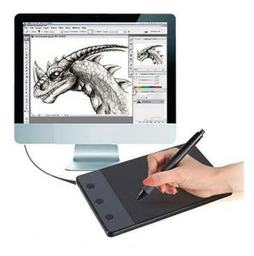
Digitizer is a computer input device that has a flat surface and usually comes with a stylus. It enables the user to draw images and graphics using the stylus as we draw on paper with a pencil. The images or graphics drawn on the digitizer appear on the computer monitor or display screen. The software converts the touch inputs into lines and can also convert handwritten text to typewritten words.
