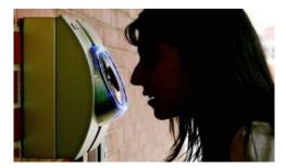
It records the voice of a person and digitizes it to create a distinctive voice print or template. The voiceprints are stored in the database, and are used to verify the voice of a person to confirm his or her identity. The person is required to speak in the normal or same voice that was used to create a voice template. It is not much reliable as it can be misused using a tape recording.
