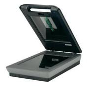
It has a glass pane and a moving optical CIS or CCD array. The light illuminates the pane, and then the image is placed on the glass pane. The light moves across the glass pane and scans the document and thus produces its digital copy. You will need a transparency adapter while scanning transparent slides.
