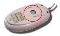
It has a system of a ball and several rollers to track its movement. It is a corded type of mouse. A mechanical mouse can be used for high performance. The drawback is that they tend to get dust into the mechanics and thus require regular cleaning.
