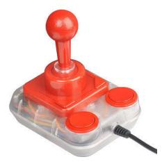
A joystick is also a pointing input device like a mouse. It is made up of a stick with a spherical base. The base is fitted in a socket that allows free movement of the stick. The movement of stick controls the cursor or pointer on the screen.
