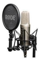
It is designed for audio recording and has a very sensitive and flat frequency response. It has a front plate called diaphragm and a back plate parallel to the front plate. When sound hits the diaphragm, it vibrates the diaphragm and alters the distance between the two plates. The changes in distance are transmitted as electric signals.
