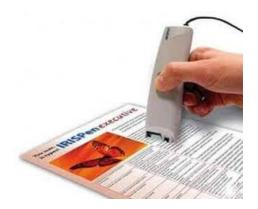
OCR computer input device is designed to convert the scanned images of handwritten, typed or printed text into digital text. It is widely used in offices and libraries to convert documents and books into electronic files.
