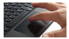
It is usually found in laptops as a substitute for the mouse. It allows you to move or control the cursor on the screen using your finger. Just like a mouse, it also has two buttons for right and left click. Using the touchpad, you can perform all the tasks that you do with a mouse, such as selecting an object on the screen, copy, paste, delete, open a file or folder, and more.
