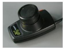
It is a simple input device that is widely used in games. It is a wheel that is held by hand and looks like a volume knob on a stereo that is used to increase or decrease the volume. Paddle moves or controls cursor or any other objects in the game in a back-and-forth motion. It is widely used as an alternative to the joystick. Besides this, the term paddle also refers to many handheld devices designed to control a function in an electronic device, computer, etc.
