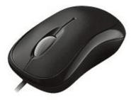
An optical mouse uses optical electronics to track its movement. It is more reliable than a mechanical mouse and also requires less maintenance. However, its performance is affected by the surface on which it is operated. Plain non-glossy mouse mat should be used for best results. The rough surface may cause problems for the optical recognition system, and the glossy surface may reflect the light wrongly and thus may cause tracking issues.
