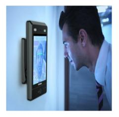
It is designed to identify a person by scanning his or her face. It takes the face measurements of a person. For example, the distance between eyes, nose, and mouth, etc., accordingly, it confirms the identity of a person. Besides this, it is smart enough to differentiate between a person's picture and the real person.
